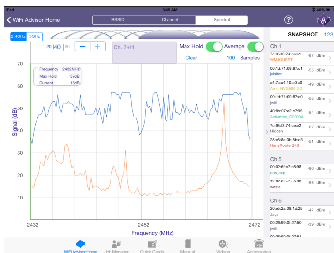
Spectral view shows interference within a channel
